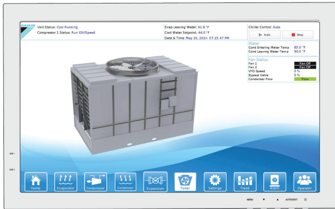
Figure 38: Cooling Tower Information
