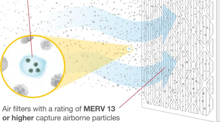
Air filters with a rating of **MERV 13 or higher** capture airborne particles between 0.3 and 1.0 microns.
