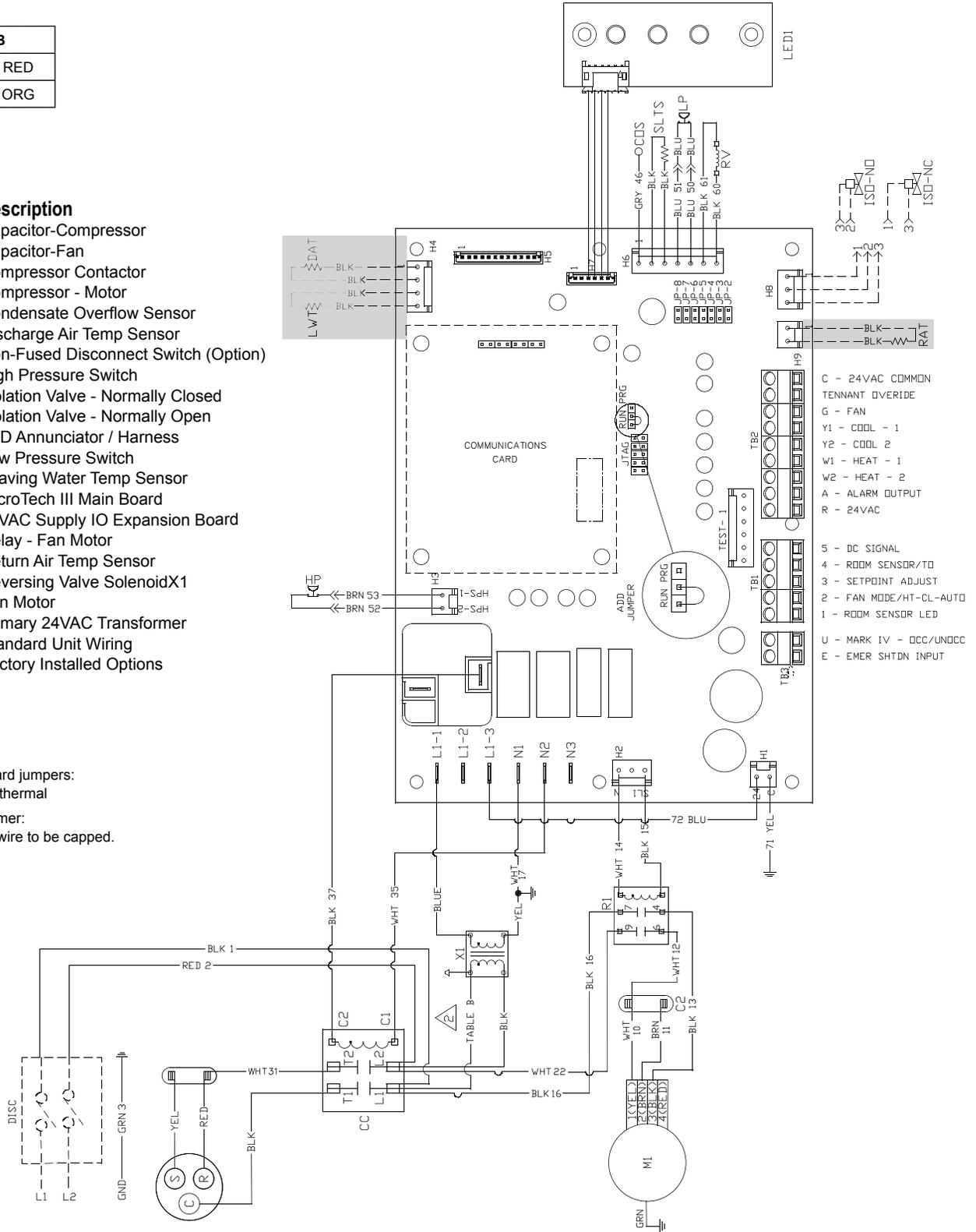
**Note:** Gray tint areas in wiring diagram: Units configured with a communication module include a Leaving Water (LWT), Discharge Air (DAT) and a Return Air (RAT) Temperature sensor. The DAT and RAT sensors are shipped loose inside the control box for field installation.
