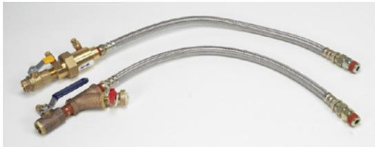
Hose kits with standard flexible supply and return hoses are recommended between the water source heat pump unit and building's hard piping system. This is to control possible noise and transmission of vibration from the unit in the space.
