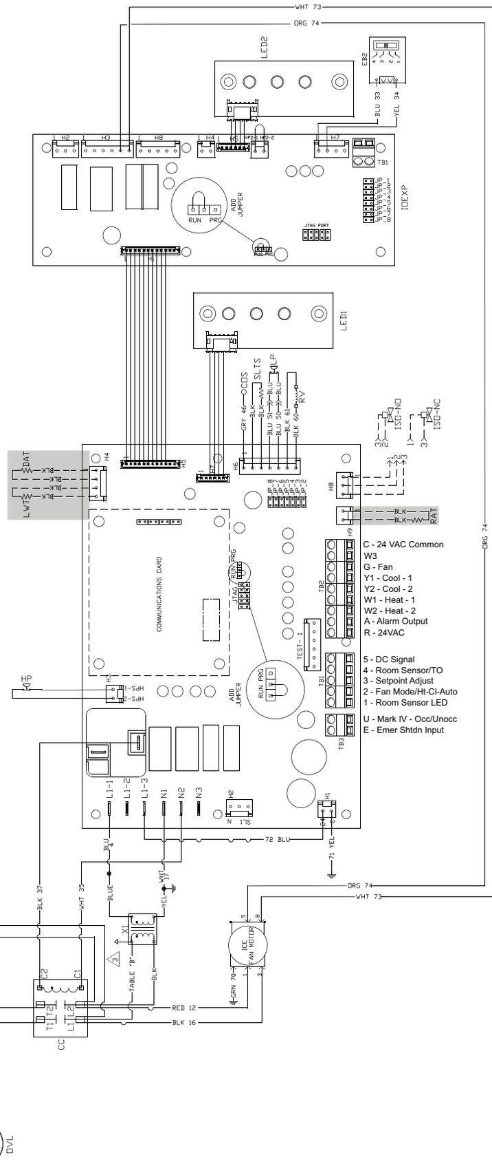
Note: Gray tint areas in wiring diagram: Units configured with a communication module include a Leaving Water (LWT), Discharge Air (DAT) and a Return Air (RAT) Temperature sensor. The DAT and RAT sensors are shipped loose inside the control box for field installation.
