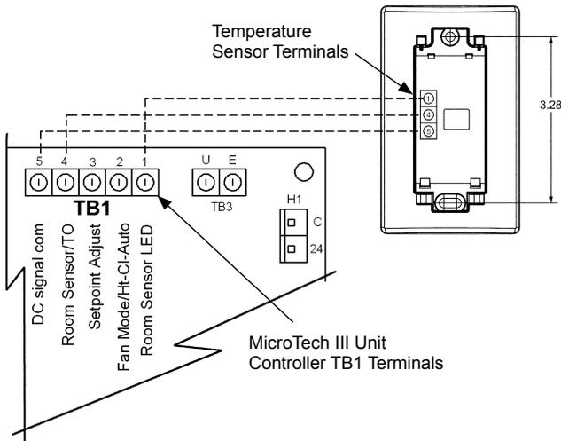
**Accessory Remote Room Sensors – Wiring (Part No.667720401 & 107096001)**
