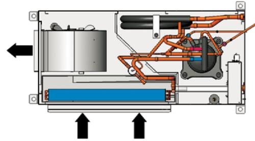
**Figure 2: Left hand return with straight discharge**
