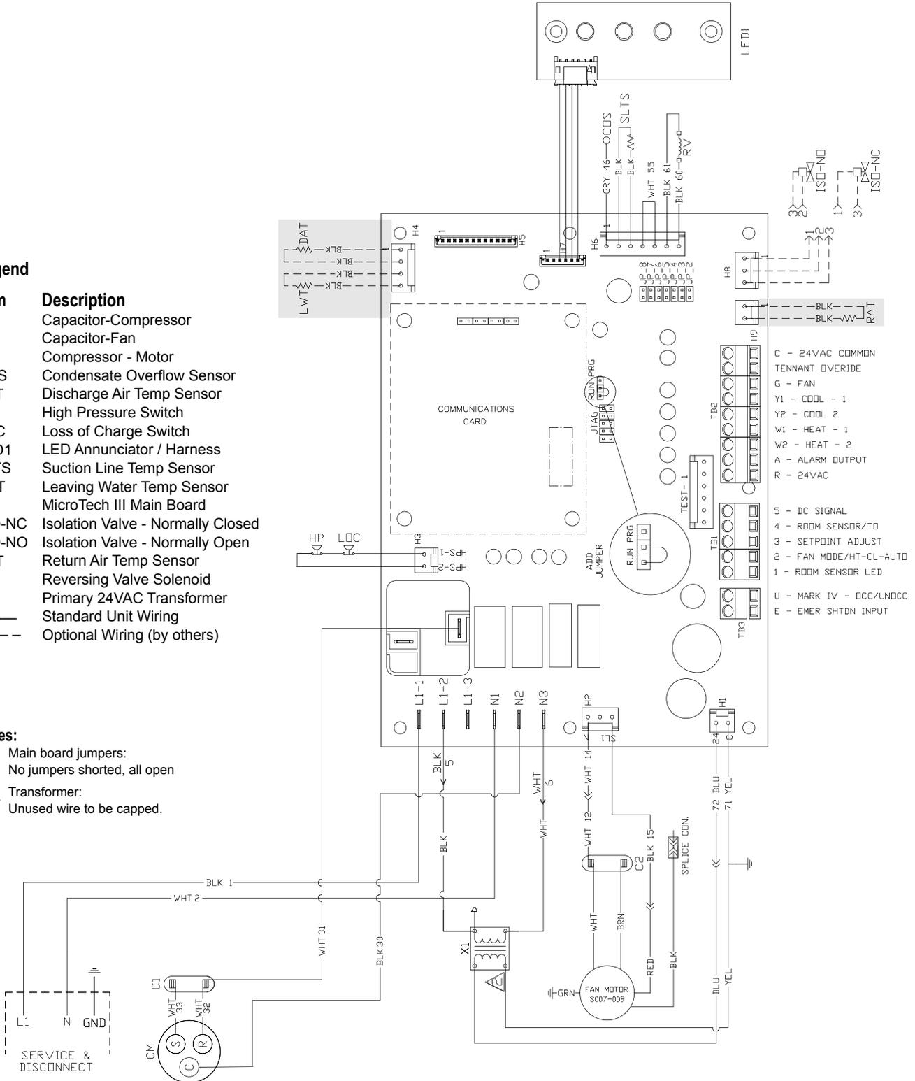
**Note:** Gray tint areas in wiring diagram: Units configured with a communication module include a Leaving Water (LWT), Discharge Air (DAT) and a Return Air (RAT) Temperature sensor. The DAT and RAT sensors are shipped loose inside the control box for field installation.
