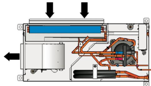
**Figure 4: Right hand return with straight discharge**
