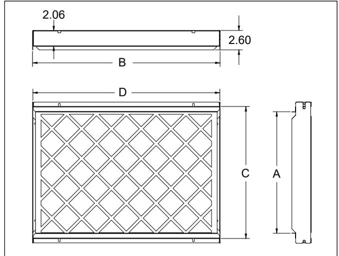
Figure 33: Optional 4" filter rack dimensions
