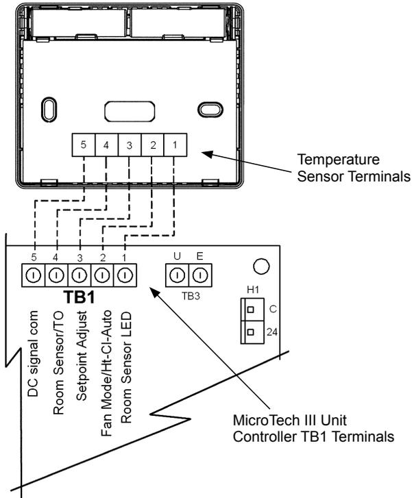
**Temperature Sensor Wiring to MicroTech III Unit Controller – P/N 669529001**
