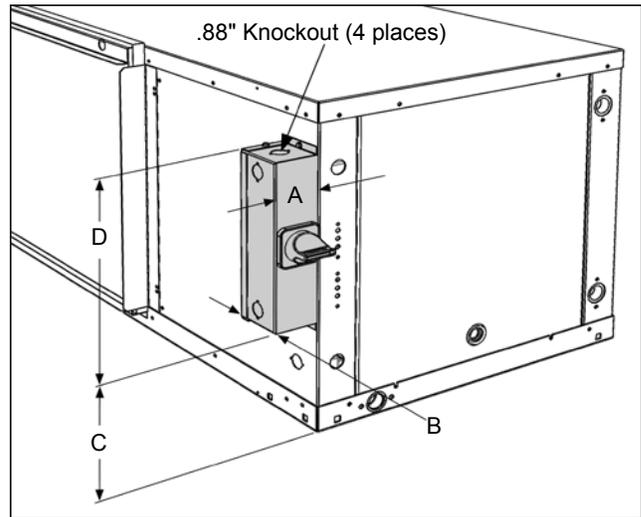
**Figure 36: Knockout locations – sizes 015 through 070**
